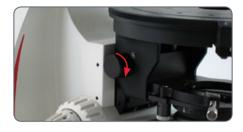
3. Swing the polarizer, which is connected to the bottom of the condenser mount, to the left.
